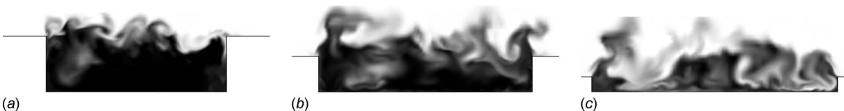
Fig. 22 Instantaneous temperature contours of eddy simulation ( BR=1 ) at x -normal planes. Top left: x=4 , top right: x=6 , and bottom: x=8 .
