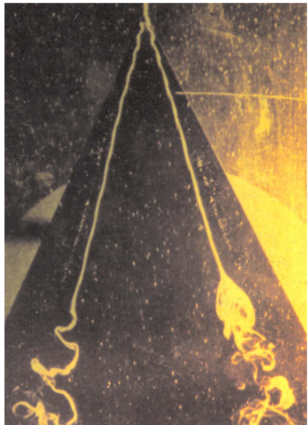
Fig. 3 Vortex breakdown above a delta wing, spiral-type on the left and bubble-type on the right [1]
